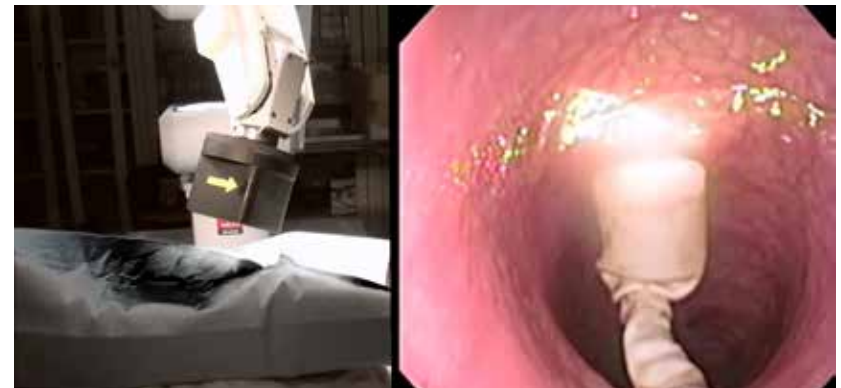
A magnet-guided camera, left, performs a 180° retroflexion, right, on a pig without internal cables or the need to push off the colon wall.
